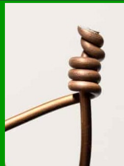
When one wire wraps around the other, the wires may slip.
