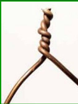
Uneven twists can apply pressure unevenly and weaken the wire.
